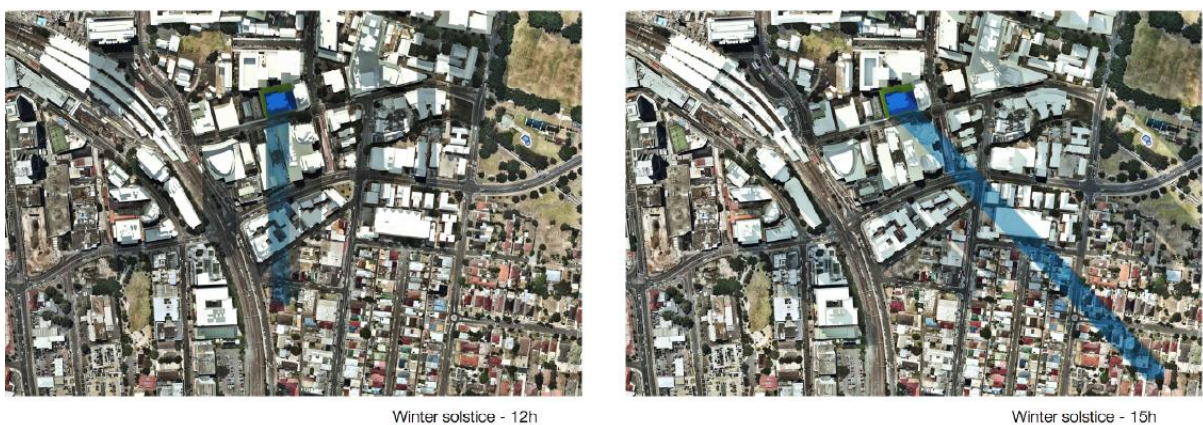
Figure 5: Overshadowing diagrams at 12pm and 3pm in midwinter, demonstrating the potential of the subject building to overshadow the residential areas to the south of the CBD. This does not consider the cumulative impact of the broader redevelopment of this locality.
